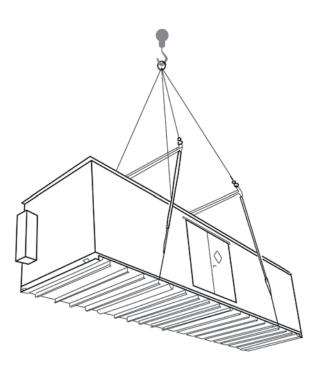
Determine the final weight of your specific building with your sales engineer (weights will vary due to specific accessories and components unique to each situation). When you arrange for off-loading with a professional crane company, be sure to notify them of the exterior dimensions (L x W x H) and weight of your building.
