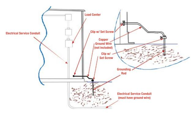
NOTE: Your grounding rod is attached to the steel grate flooring during shipment of your building.
