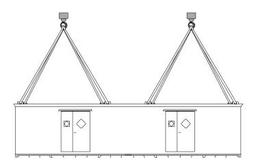
**Note:** When you arrange for off-loading with your crane company, be sure to notify them of the exterior dimensions ( $L \times W \times H$ ) and weight of building.
